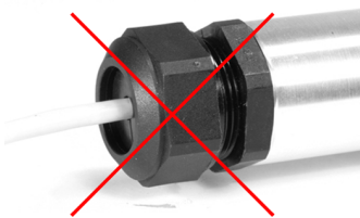
Figure 9: Improper sealing: too loosely tightened, no compression of the rubber
