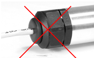
Figure 10: Improper sealing: overtightened, too much compression of the rubber
