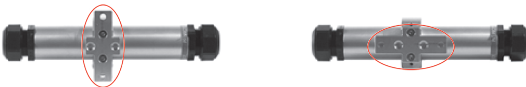
Figure 4: Mounting the bracket on the protector - lateral and longitudinal alignment
